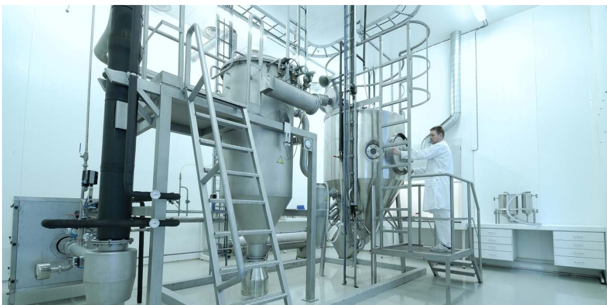
Spray-drier at the manufacturing plant for Medox®
