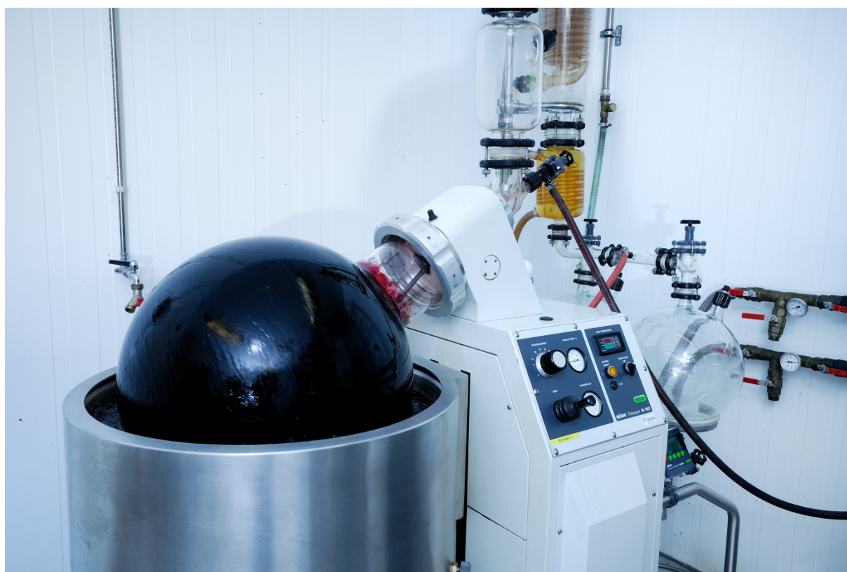
One of the Rotavapors used in an early generation of our patented Medox ® manufacturing plant is still in use.
