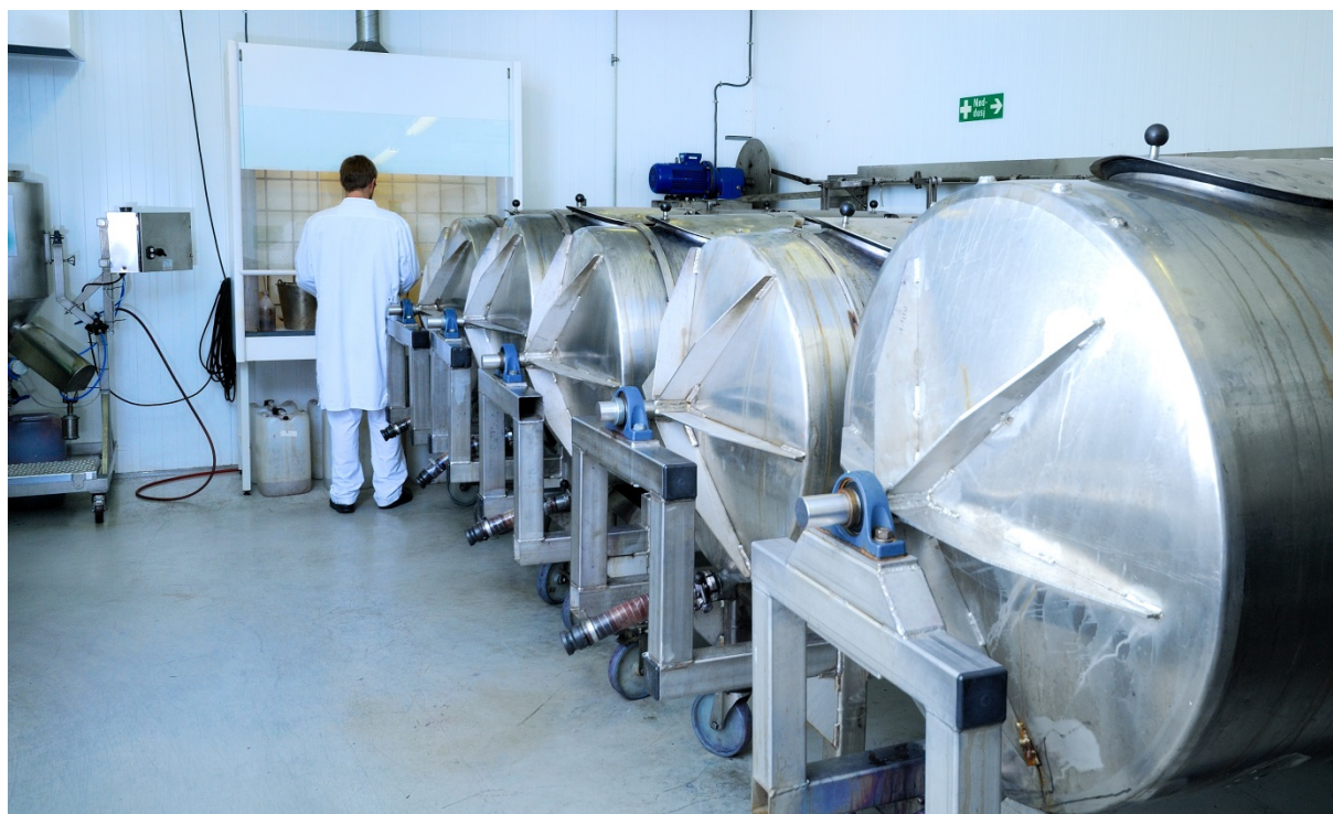
Bilberry and black currant skin dissolved in tanks before being moved to the next step in our patented manufacturing.
